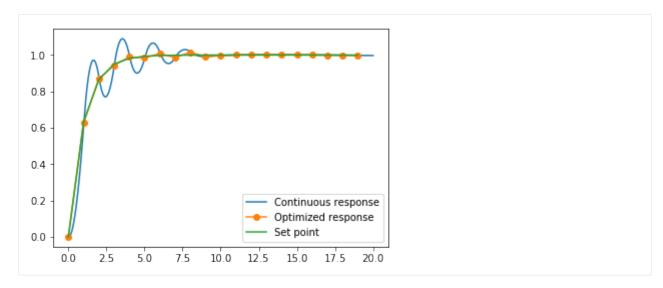
One of the reasons for the popularity of MPC is how easy it is to change its behaviour using weights in the objective function. Try using this definition instead of the simple one above and see if you can remove the ringing in the controller output.
