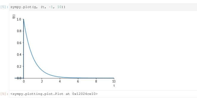
Earlier, we calculated the step response of the system by calculating  $U(s) = \frac{1}{s}$ , therefore  $Y(s) = \frac{G(s)}{s}$  and then calculating the inverse Laplace:
