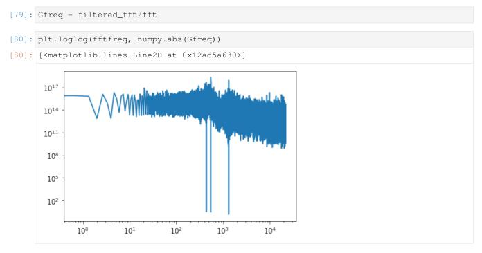
The gain is a bit strange (very large) here because we used a pure sinusoidal signal to start with, with no low frequency content, but we can still see the characteristic shape of a first order transfer function.
