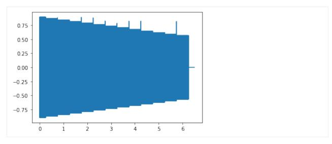
When we zoom in so that we can see the wave forms, we can see that the low frequencies are attenuated less than the high frequencies.
