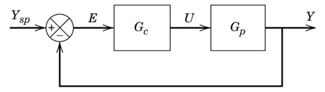
Let's derive the closed loop transfer function. There are three equations represented in the above diagram:
