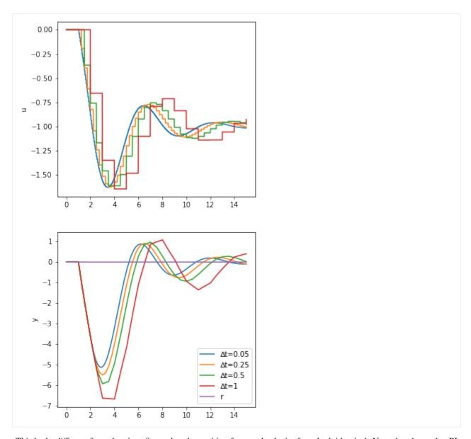
This looks different from the given figure, but the position form and velocity form look identical. Note that the analog PI controller gets better results than the digital approximations with the same controller parameters. "Better" in this context means that in general the error is smaller (note the worst case error in the analog case is about 5, while in the digital case it's almost 7.
