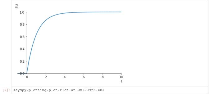
We can get the same result by convolving the unit step function with the impulse response. Sympy doesn't handle the improper integral correctly here (as of the below version number):
