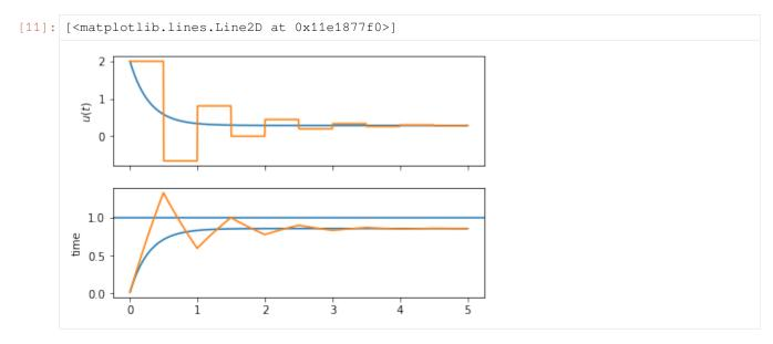
Notice the difference? Because the discrete controller only calculates its values at the sampling points and because the ZOH keeps its output constant, the discrete controller takes more action later on, in fact introducing some oscillation where the continuous controller could use arbitrarily large gain.
