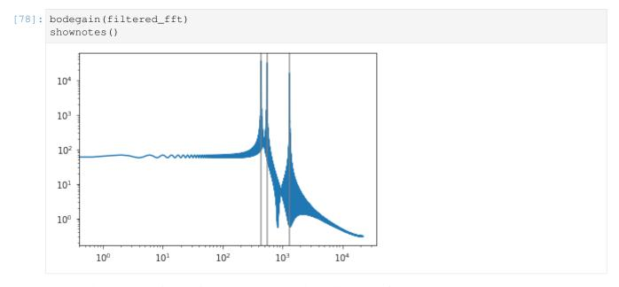
It's clear how the lower frequencies are attenuated (made smaller) by the filter.
