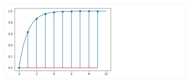
But what does it really look like between data points? First, let's construct the response of the system to a single sampling time length pulse input
