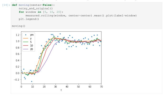
As with all causal filters (filters which only use information from *before* the point at which they calculate a value) we see that the filter introduces a delay between the original signal and the filtered signal.
