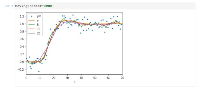
Note that these signals are much closer to the original data. As a general rule, non-causal filters outperform their causal counterparts at the cost of having to be done offline. However, also notice that the wider windows are making the response look less sharp at the start and suppressing the overshoot.
