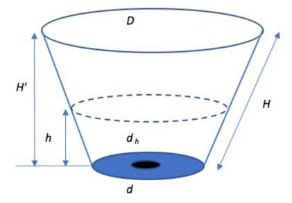
D and d are the top and bottom diameters of the cup, H is the side length between the diameters,  $d_h$  is the hole diameter. We also define H' as the vertical height of the cup and h as the vertical height (or level) of the liquid in the cup
