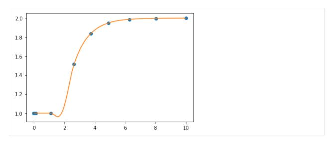
That downward bump in the level is a numerical anomaly due to the places where the samples are taking during integration. To make sure that we don't miss the moment when the step occurs, we can limit the step size that <code>solve\_ivp</code> uses.
