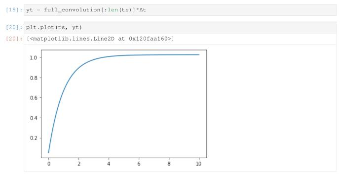
Notice that this allows us to calculate the response of a system to an arbitrarily complex input numerically. It also gives us a whole new way to think about how a system will behave by thinking about what its impulse response looks like.
