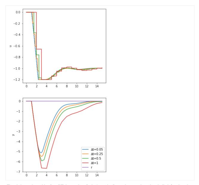
The windup on the position form PID is very clear. In the "wound up" case, the output is stuck at the limit for a long time as the controller has to unwind the integral before moving away from the limit. In the velocity form, the output comes away from the limit much faster.
