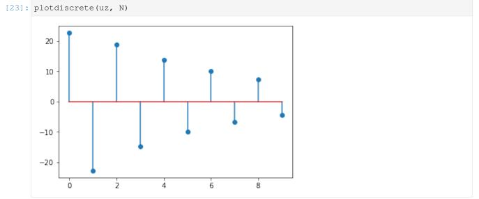
This oscillating controller output is known as "ringing". It is an undesirable effect.
