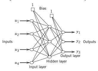
Each circle represents a neuron, and the output of the neuron is calculated as shown below. In simple terms, the output of a neuron is the weighted average of its inputs, passed through what is known as an activation function. The function shown in the picture is known as a logistic or sigmoid function.
