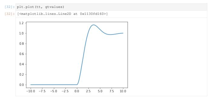
Now, let's try to get the same answer by exploiting the frequency response of the transfer function. First, we need a function which can evaluate the transfer function at particular values and return a numeric result. As before I use lambdify and the extra argument to make the function able to work with numpy arrays
