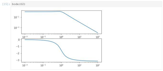
It is easy to predict how the product of the two functions would look since both plots add together when the transfer functions are multiplied.
