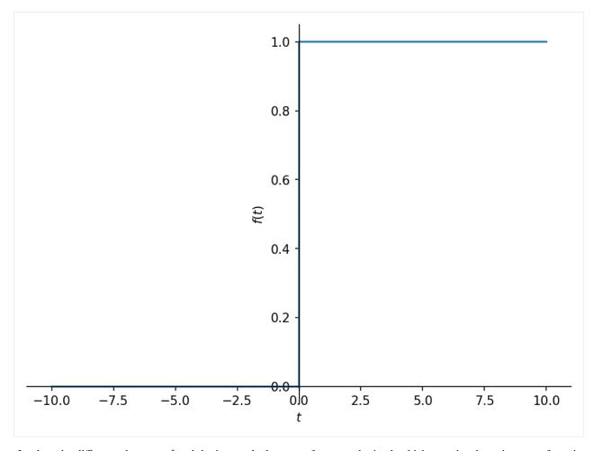
Look at the difference between f and the inverse laplace transform we obtained, which contains the unit step to force it to zero before t=0.
