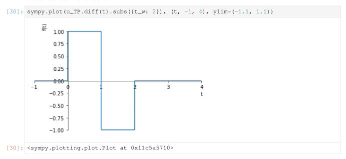
We now see that the derivative of a piecewise linear continuous function is a piecewise constant function. We can apply our rule for piecewise constant functions and integrate the steps to ramps:
